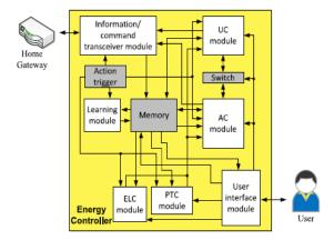
Fig. 2. The components of the Home energy control system (in the cloud server).
