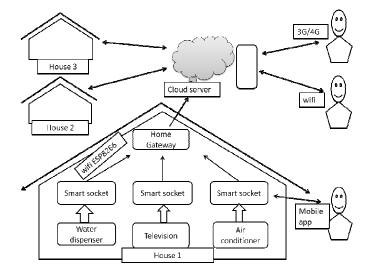
**Fig. 1.** The IoT based system architecture of home energy control system.
